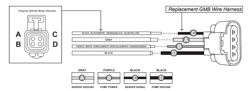
NOTE: Crimped connectors must be staggered to allow the harness to fit inside the vehicle wire sleeve.
